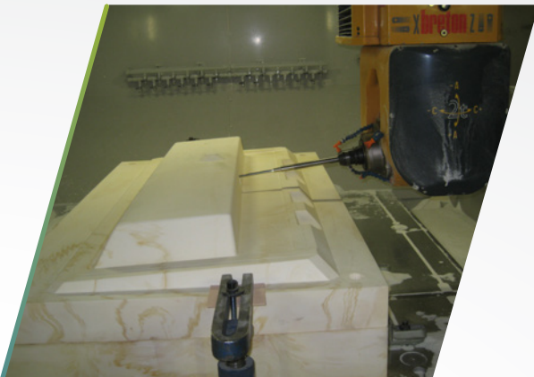
2-part CAM-tooled resin mould
